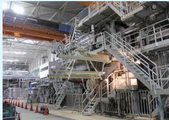
State-of-the-art household paper manufacturing machine
