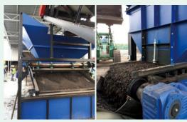
PKS being loaded into a receiving hopper by heavy machinery
